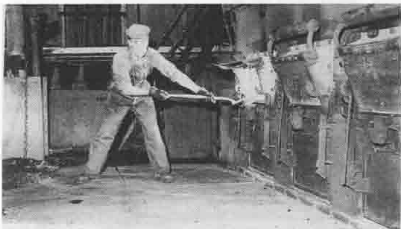
Fig. 6: Paul Stuber as a fireman on the William J. Filbert, firing up a boiler with 50 pounds of coal a minute.
