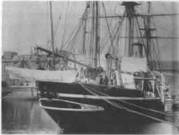
*HMS Condor* was a barque-rigged twin screw steel steam sloop. Although some sources give her rig as barquentine or brigantine a photo of the ship, first of her class, shows that she was barque rigged. Sisterships were later rigged as barquentines or brigantines to reduce sail area after the loss of *Condor*; all had their sailing rig removed within a few years. She was a new ship, having been launched at Sheerness in December 1898 and
