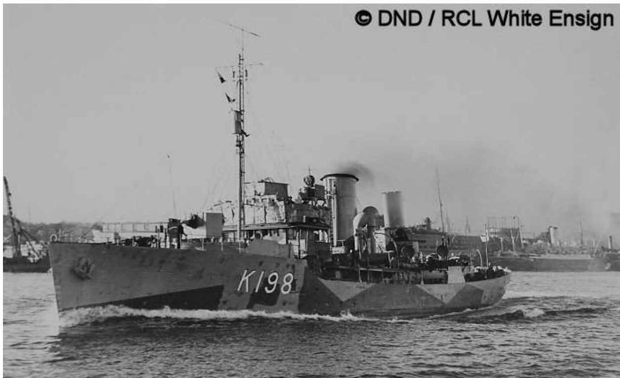
Figure 2: HMCS Spikenard approximately two months before being torpedoed. Note the splinter mats on bridge railings, wood monkey island, and the SW-1C radar antenna at the top of the mast. Credit: Dept. National Defence of Canada #MC-2975.
