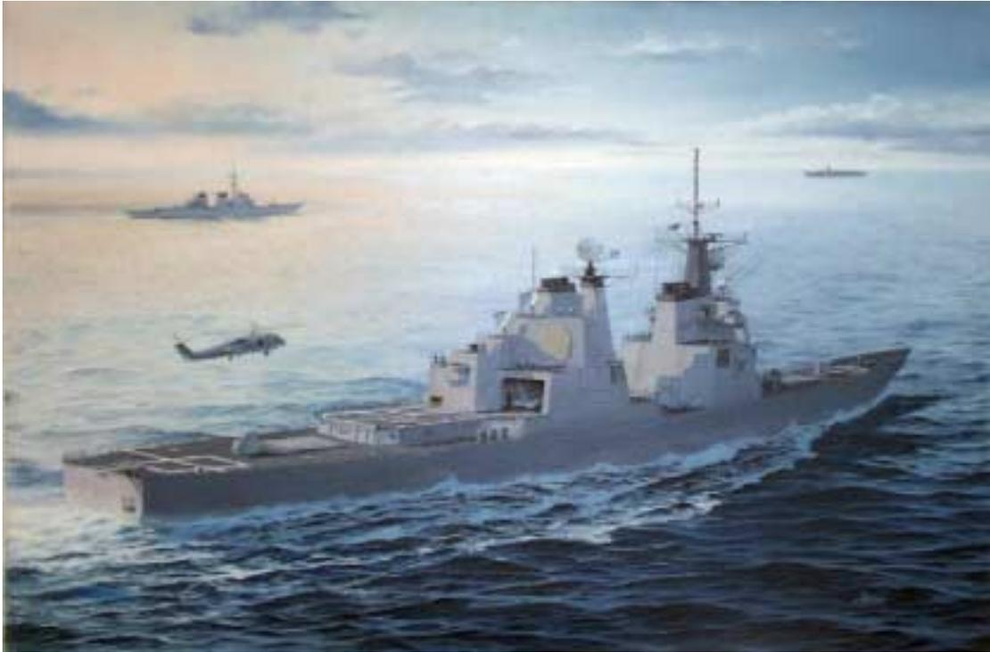
**Figure 26 CGBL; a CG 47 combat system but with the hull features of a DDG 51, weapons systems modularity and increased service life reerves**
