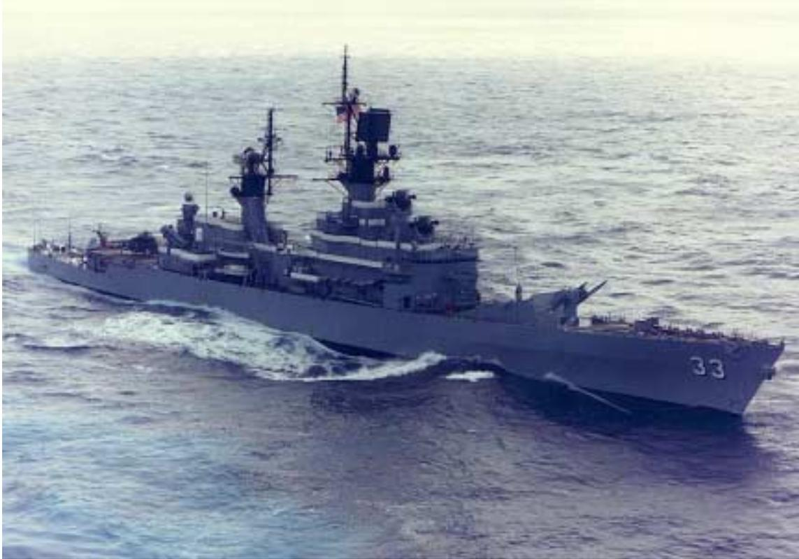
**Figure 22 *Belknap* Class *USS Fox* (CG 33) after installation of Harpoon and CIWS.**
