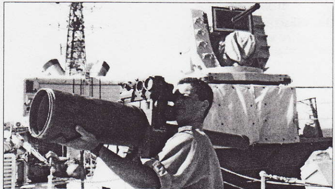
New systems fitted in Athabaskan included Javelin missiles (foreground) and the Phalanx CIWS for missile defence.
