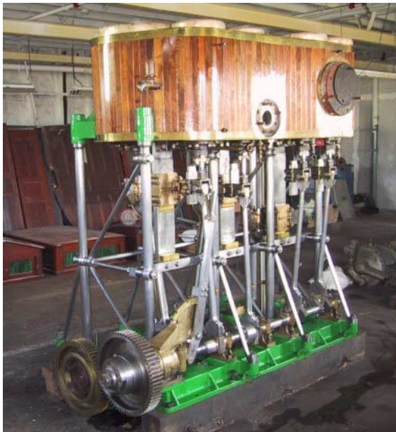
The original J.W. Sullivan steam engine with varnished lagging, polished brass and steel.
