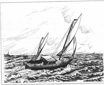
Note the able form of the underbody, the shipshape appearance of the profile and particularly the use of the good old gaff rig. The engine is a Sterling Chevron developing 100 h.p. and it is expected that she will shove along at 10 knots in spite of the ballast, the 400 gallons of gasoline and the 250 gallons of water.
