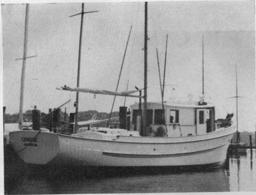
Chinook rightly needs another ton of ballast. Here she's shown with all tanks full
