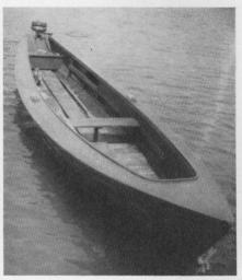
the seams are caulked. Construction is on the heavy side, resulting in a workboat capable of withstanding much abuse.
