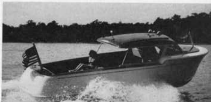
Richardson 25 foot semienclosed Utility, speed 17 to 30 miles an hour depending on power installation. Banks nicely on turns in very small radius. Molded mahogany construction over white oak frames, stem and keel
