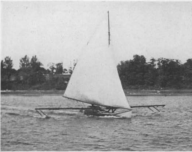
The sailplane on a close reach. It will be noted that she sails without any angle of heel.
