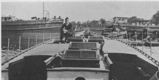
Engine room entrance on port, cabin companionway to starboard.
