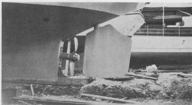
Reversible propeller with blades turned in neutral position.
