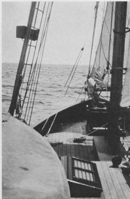
"Mahdee" has a sunken deck forward and is flush from rail to rail amidships
