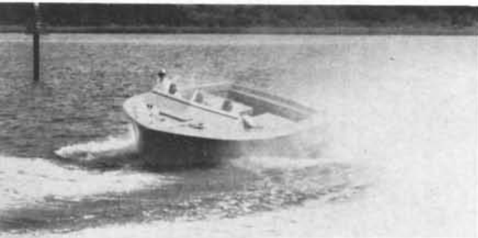
Hatteras prototype hull hits a hard-over turn at full throttle. Unobstructed bottom permits hull to quickly reverse direction
