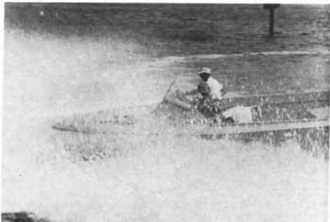
Slane demonstrates crash stop capability by reversing jet pumps when moving forward at full speed
