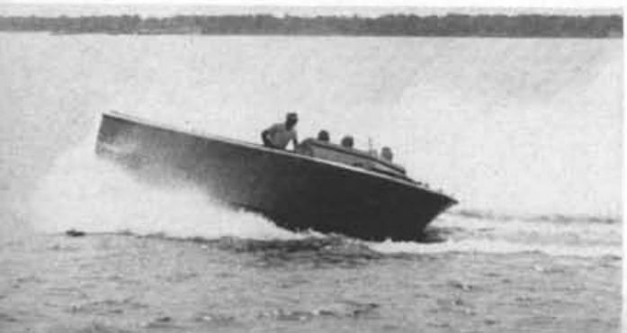
Hatteras prototype hull hits a hard-over turn at full throttle. Unobstructed bottom permits hull to quickly reverse direction
