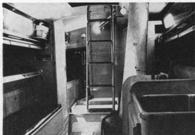
Looking aft from galley: Padded bunk board on semi-circular track (left) locks up for sleeping or down to be backrest for seat
