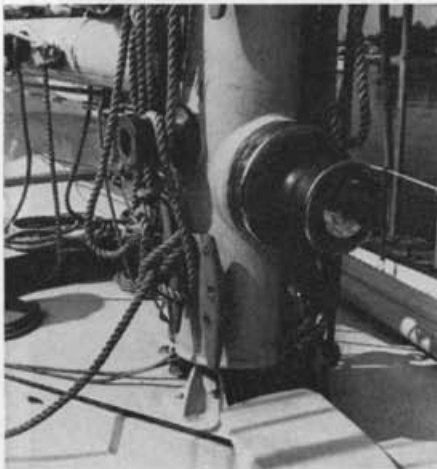
To avoid high weight, winches are mounted low on mast which is stepped on deck in unusual manner
