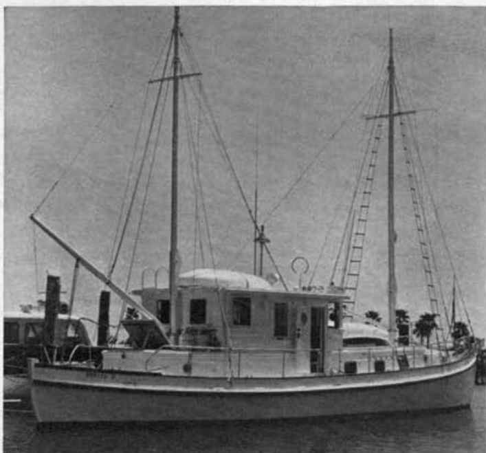
"Bonita's" spread-out sail rig is effective. Both masts are hinged to permit easy lowering
